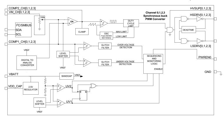
Figure 3 –SMB113A/B and SMB117/A internal block diagram. Programmable functional blocks include: level shifters, digital to analog converter and the VM\_CH[0,1,2,3] voltage dividers.
