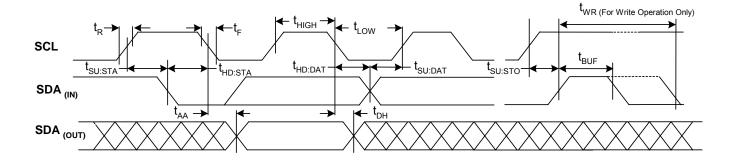
Figure 4 – I<sup>2</sup>C timing diagram
