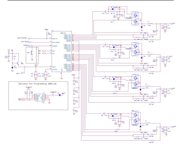
Figure 9 – Applications schematic showing SMB113A operation from a +12V input supply.
