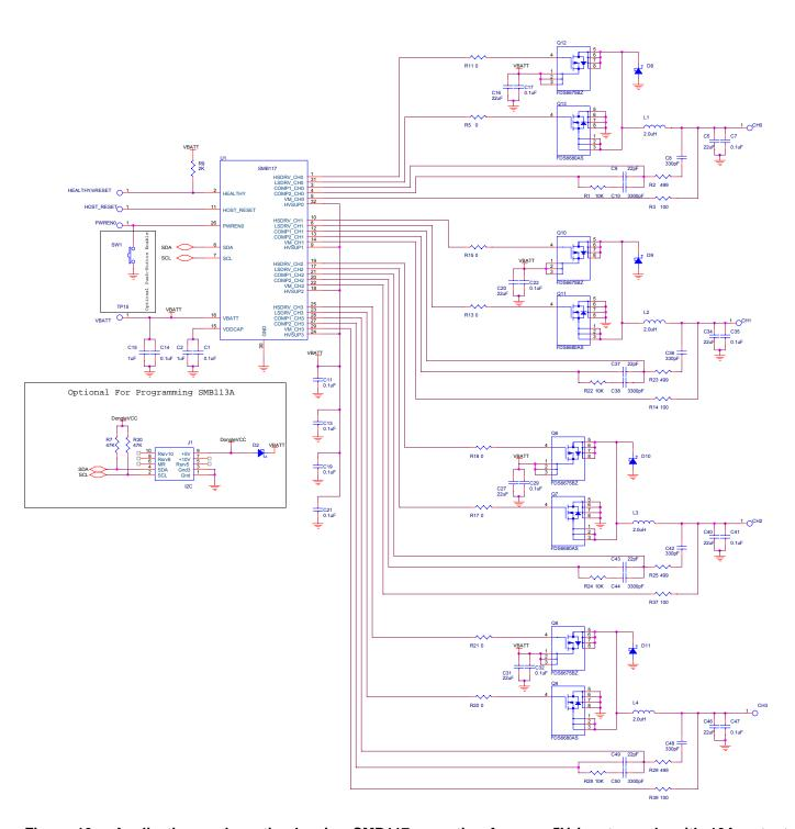
Figure 10 – Applications schematic showing SMB117 operation from a +5V input supply with 10A output current capability.
