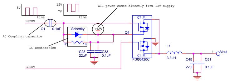
Figure 7 - High-voltage operation
