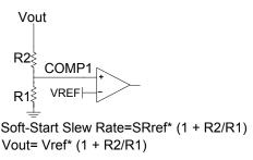
Figure 6 – The output voltage is set by the voltage divider. The VREF voltage is programmable from 0 to 1.0 volt in 4mV increments via the I<sup>2</sup>C interface
