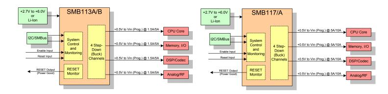
Figure 1 – Applications schematic featuring the SMB113A/B/117/A programmable DC-DC controllers.
