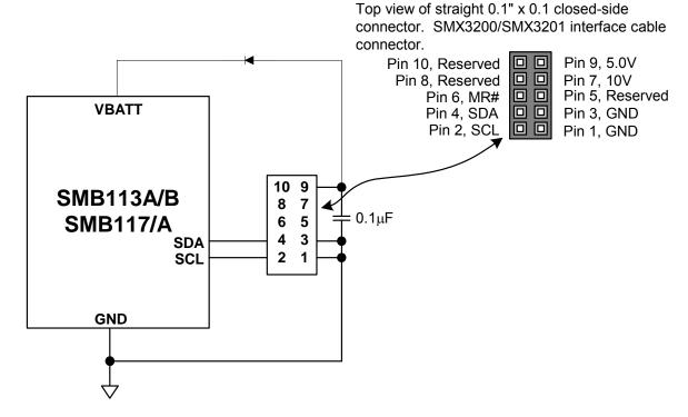
Figure 11 – SMX3200/SMX3201 Programmer I<sup>2</sup>C serial bus connections to program the SMB113A/B or SMB117/A.
