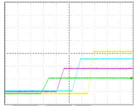
Figure 5 – Power on sequencing waveforms.
